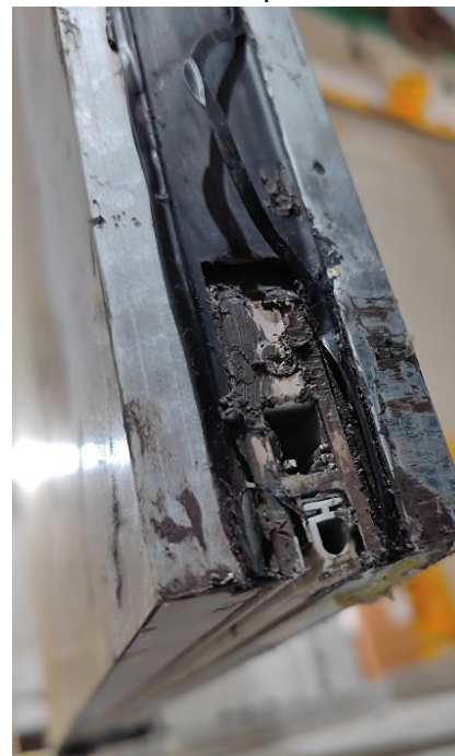
Photo 29 - The bottom edge of inactive leaf after medium temperature test
