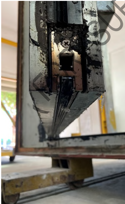
Photo 13 - The bottom edge of active leaf after medium temperature test
