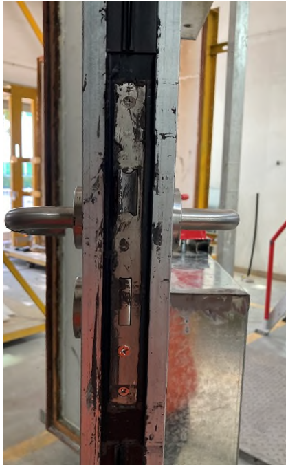
Photo 11 - The meeting edge of active leaf after medium temperature test
