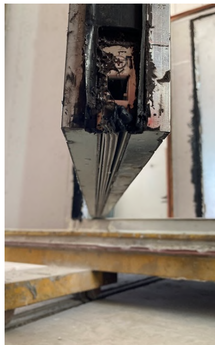
Photo 10 - The bottom edge of door leaf after medium temperature test
