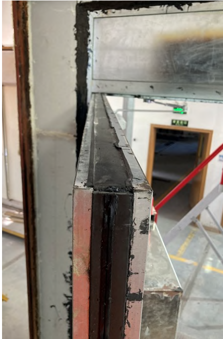
Photo 7 - The top edge of active leaf after medium temperature test
