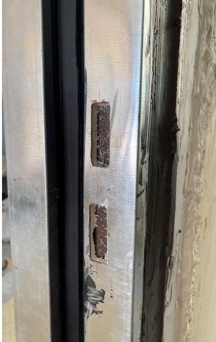
Photo 7 - The position of strike plate after medium temperature test
