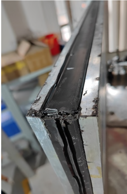
Photo 22 - The top edge of active leaf after medium temperature test
