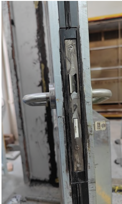
Photo 26 - The meeting edge of active leaf after medium temperature test
