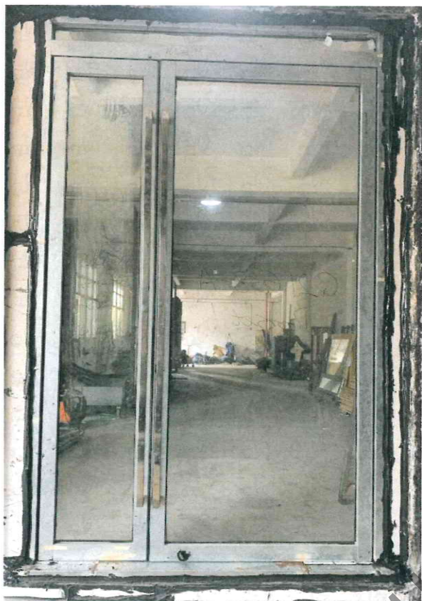
Photo 1: Exposed face of Doorset before the test.
