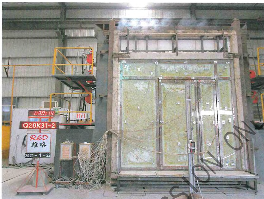
Photo 3: The unexposed face of the specimen a heating period of 90 minutes.
