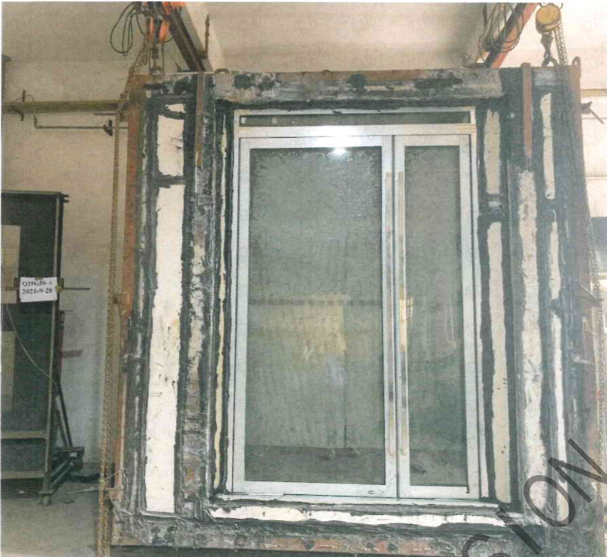
Photo 3: Unexposed face of Doorset during the test
