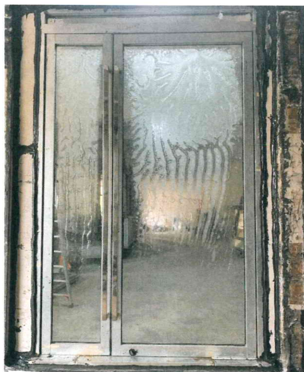
Photo 2: Exposed Face of Doorset after the test.
