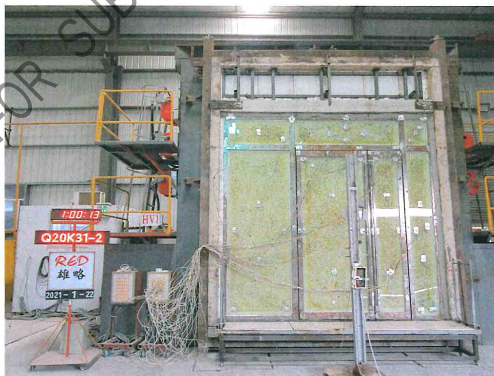
Photo 2: The unexposed face of the specimen a heating period of 60 minutes.
