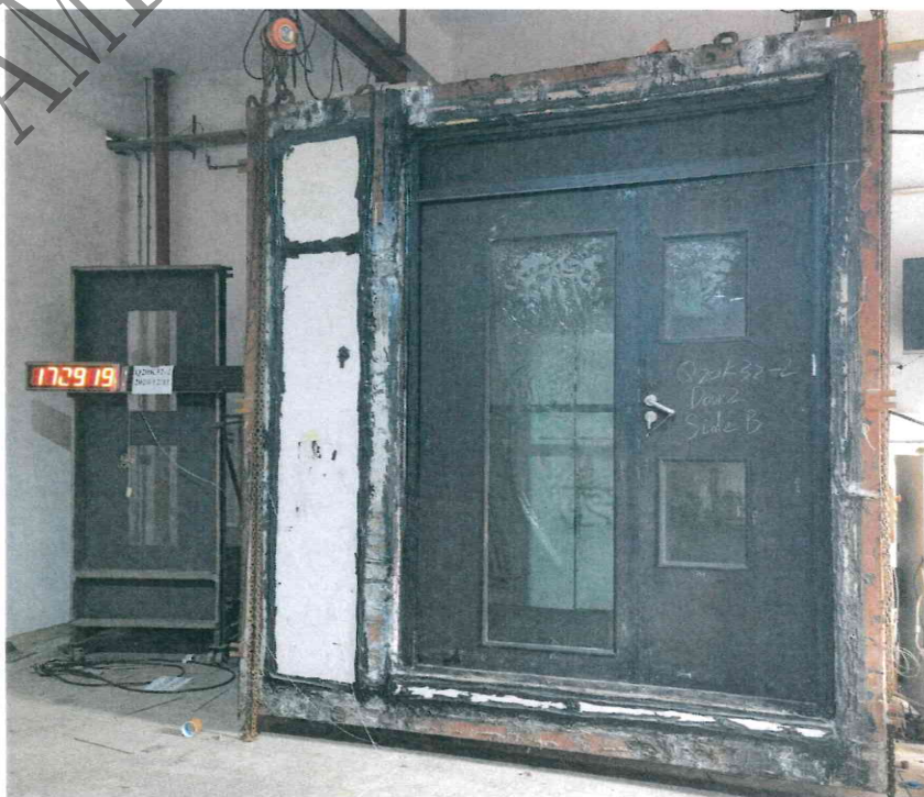
Photo 6: Unexposed face of Doorset '2' during the test
