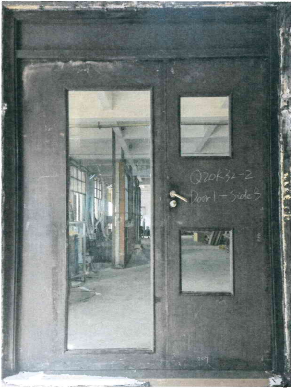
Photo 1: Exposed face of Doorset '1' before the test.
