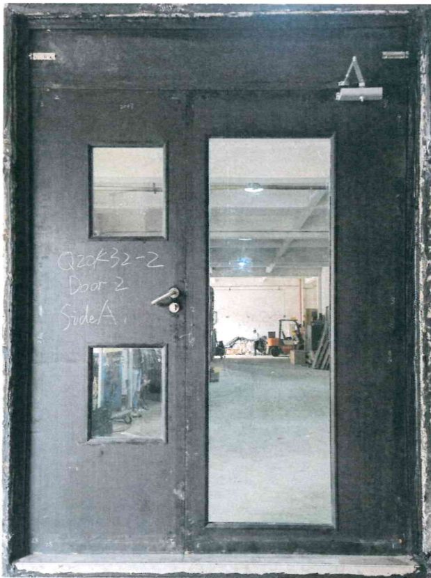
Photo 3: Exposed Face of Doorset '2' before the test
