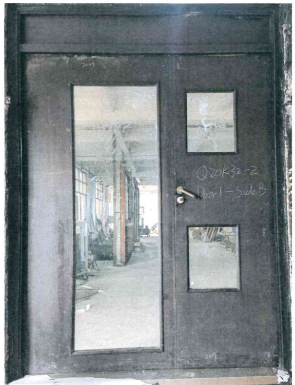
Photo 2: Exposed face of Doorset '1' after the test.
